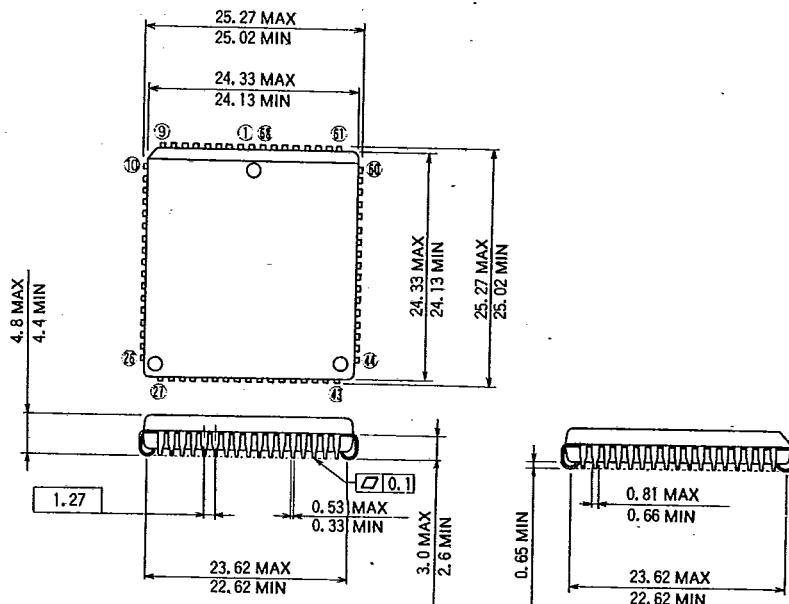
TYPE 80P6 80-PIN MOLDED PLASTIC QFP
